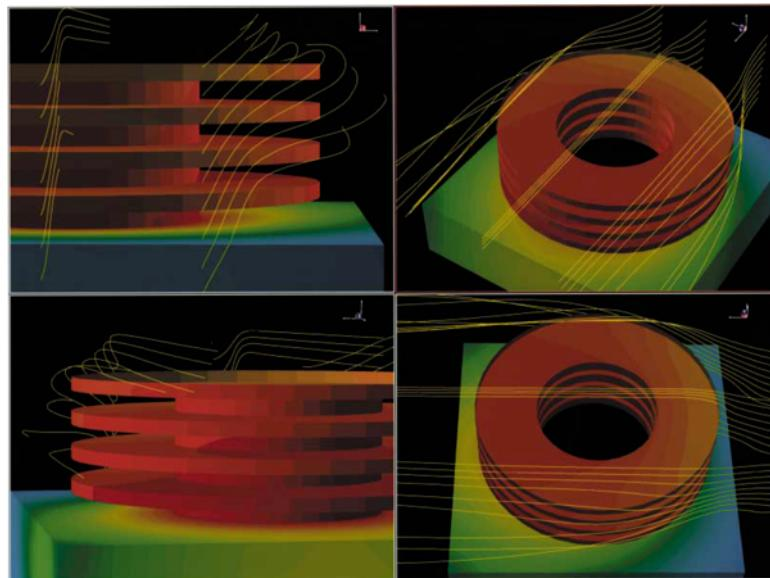
Visualization of the cooling process for an electronics module. Centric's Spectrum(TM) is used for multiphysics simulation and visualization of this thermal management application. The color contours represent the temperature field within a Motorola MCA2800-ALS bipolar gate array. Streamlines of the cooling flow around the module are also shown.
